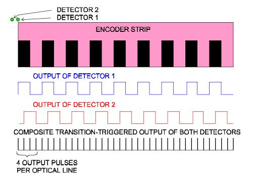
Figure 2-8. Quadrature Signal Generation.
